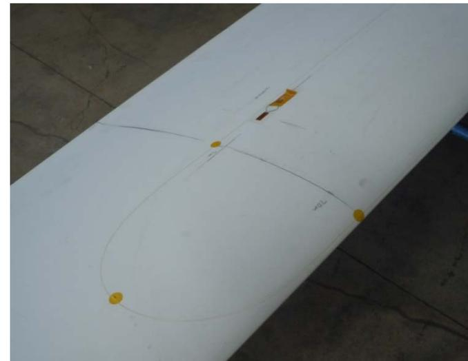
*An HD-FOS sensor bonded to the surface of the turbine blade*
